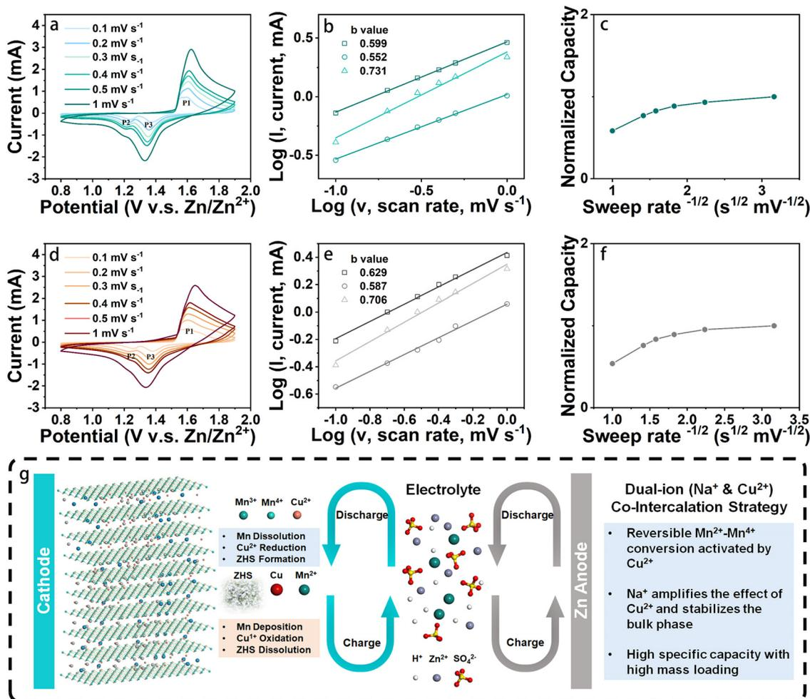
Fig. 4 (a) and (d) CV curves with scan rates ranging from 0.1 to 1 mV s<sup>-1</sup>, (b), (e) diffusion-capacitive control contribution, and (c) and (f) the relationship between normalized capacity and sweep rate of NCMO and NMO, respectively. (g) Schematic diagram illustrating the charge and discharge process of NCMO cathodes in ZIBs.
