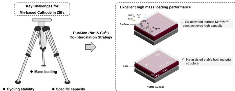
**Scheme 1** Schematic representation of the manganese oxide cathode based on a dual-ion co-intercalation strategy that simultaneously boosts surface  $\text{Mn}^{2+}/\text{Mn}^{4+}$  two-electron transfer and maintains the stability of the host material structure to cope with the key challenges of mass loading, cycling stability, and specific capacity in Mn-based cathodes.
