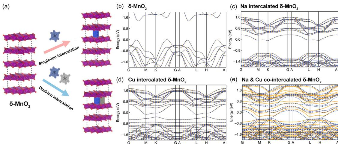
**Fig. 1** (a) Ion intercalation strategy for high performance  $\delta\text{-MnO}_2$  cathode materials and band structures of (b)  $\delta\text{-MnO}_2$ , (c) Na intercalated  $\delta\text{-MnO}_2$ , (d) Cu intercalated  $\delta\text{-MnO}_2$  and (e) Na & Cu co-intercalated  $\delta\text{-MnO}_2$  based on DFT modelling.
