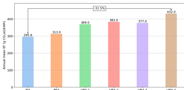
Fig. 2 Annual mean grid emission factor for Germany in 2020, according to different sources (IEA, 6,7 EEA 8 and UBA 9 ). UBA 1–UBA 4 represent four different approaches to calculating a grid EF, varying the aspects impact metric (CO 2 , CO 2 -equivalents), inclusion of electricity trade (with, w/o) and system boundaries (direct, life-cycle emissions). UBA 1: CO 2 , w/o trade, direct emissions; UBA 2: CO 2 , with trade, direct emissions; UBA 3: CO 2 e, w/o trade, direct emissions; UBA 4: CO 2 e, w/o trade, life-cycle emissions.
