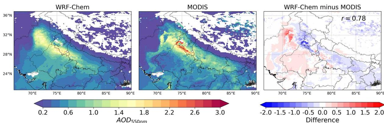
Fig. 3 Modelled and MODIS retrieved  $\text{AOD}_{550\text{nm}}$  sampled at overpass times of 10.30 (Terra) and 13.30 (Aqua) and averaged over the pollution episode. The right panel shows the absolute differences between the model and satellite values (with a % difference plot shown in Fig. S6†), and  $r$  is the Pearson's correlation coefficient.
