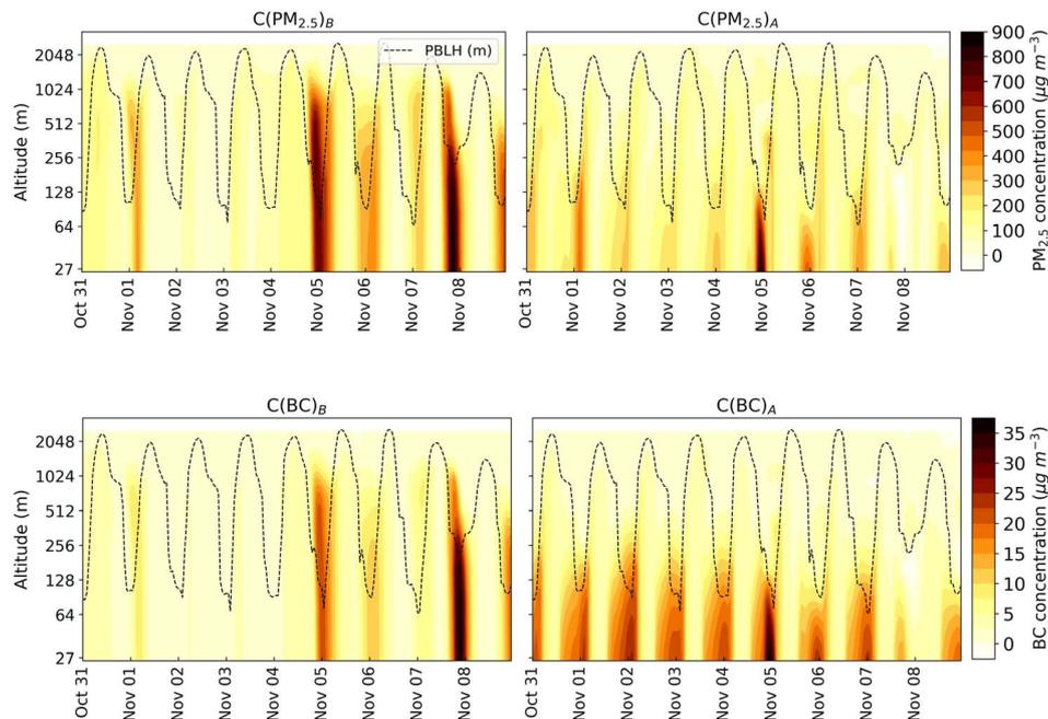
Fig. 9 Modelled vertical evolution of changes in total  $\text{PM}_{2.5}$  (top) and BC (bottom) concentrations over Delhi due to the exclusion of anthropogenic and BB emissions as compared to the Base scenario during the study period. The dashed line in the top panels denotes the hourly variation of the modelled planetary boundary layer (PBL) height (identical in all sensitivity runs).
