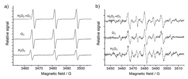
Fig. 5 EPR experimental spectra utilizing TEMP (a) or DMPO (b) as radical probes.
