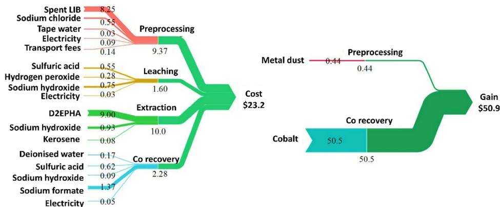
Fig. 23 Economic cost and gain breakdown for spent LIB recycling with hydrometallurgy. Reproduced with permission from ref. 210; Copyright 2023, Elsevier.
