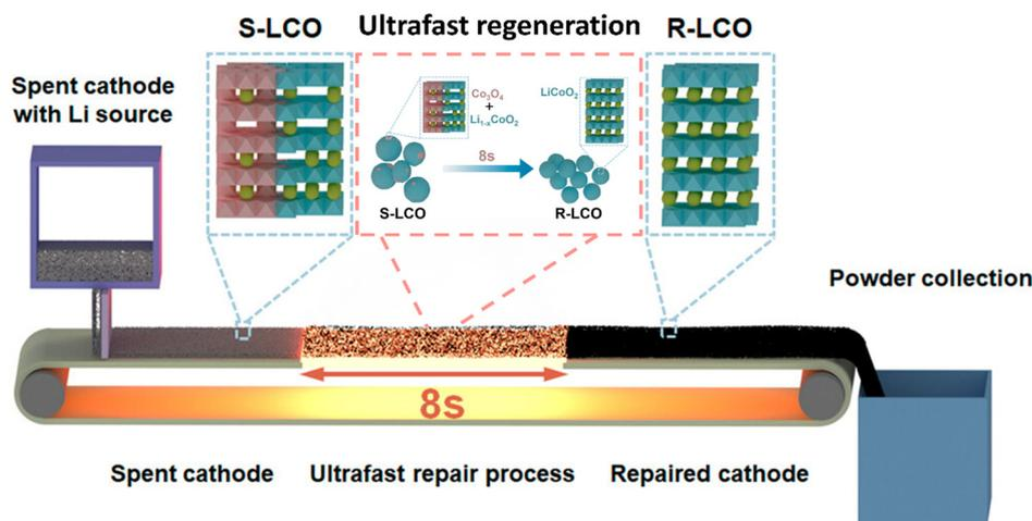
Fig. 6 Rapid Joule heating process for non-destructive reconstruction of cathodes. Reproduced with permission from ref. 81; Copyright 2023, American Chemical Society.
