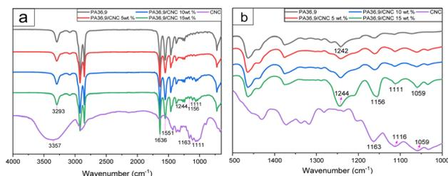
Fig. 2 FTIR spectra of PA36,9,<sup>12</sup> CNC and PA36,9/CNC nanocomposites with different CNC contents in the ranges of (a)  $4000\text{--}650\text{ cm}^{-1}$  and (b)  $1500\text{--}1000\text{ cm}^{-1}$ .
