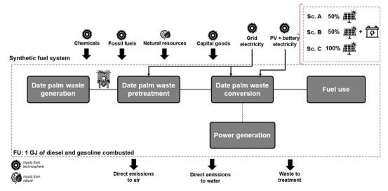
Fig. 2 Synthetic biofuel system with PV integration.
