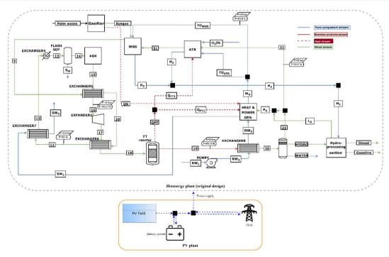
Process diagram of the synthetic biofuel production plant (grey dashed box) with PV plant integration (orange box).
