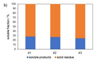
Fig. 7 (a) Amount of soluble products and (b) HPLC-chromatograms for three experiments of pre-extracted apple pomace. Reaction conditions: 6% acid content, 170 min milling duration, 500 rpm, 5 g substrate and 166.48 g zirconia balls.
