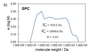
Fig. 6 Molecular weight distribution from GPC-measurement of the experiment with (a) non-extracted apple pomace and (b) pre-extracted apple pomace. Reaction conditions: 6% acid content, 170 min milling duration, 500 rpm, 5 g substrate and 166.48 g zirconia balls.
