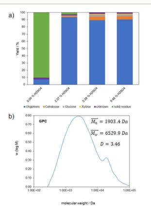
Fig. 2 (a) Composition of the product mixture after mechanocatalytic partial depolymerization with different acid contents; reaction conditions: 500 rpm, 86 min effective milling duration, 5 g substrate and 163.48 g zirconia balls. (b) Molecular weight distribution from GPC-measurement of the experiment with 2.37% sulfuric acid.
