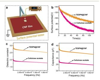
Fig. 4 (a) Schematic diagram of the surface charge test. (b) Surface charge versus time curves of cellulose acetate and TESPN@CNF films. Comparison of the (c) dielectric constant and (d) capacitance of cellulose acetate and TESPN@CNF films.
