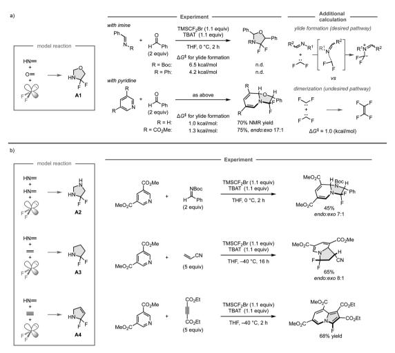
Fig. 13 Experimental realization based on computationally predicted three-component reactions. (a) Realization of the predicted reaction with the support of additional DFT calculations at the  $\omega$ B97X-D/Def2-SVP/CPCM(THF) level. (b) Further experimental demonstrations.
