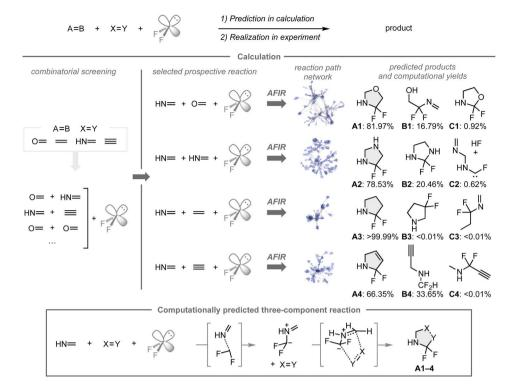
Fig. 12 Computational reaction screening with difluorocarbene for the exploration of three-component reactions. The automatic searches for the reaction pathways were performed using the AFIR method at the  $\omega$ B97X-D/LanL2DZ/CPCM(THF) level. Single-point energy calculations were performed for the obtained pathways at the  $\omega$ B97X-D/Def2-SVP/CPCM(THF) level. The top three predicted products in terms of computational yield in the reaction path network at 300 K within 1 second are shown.
