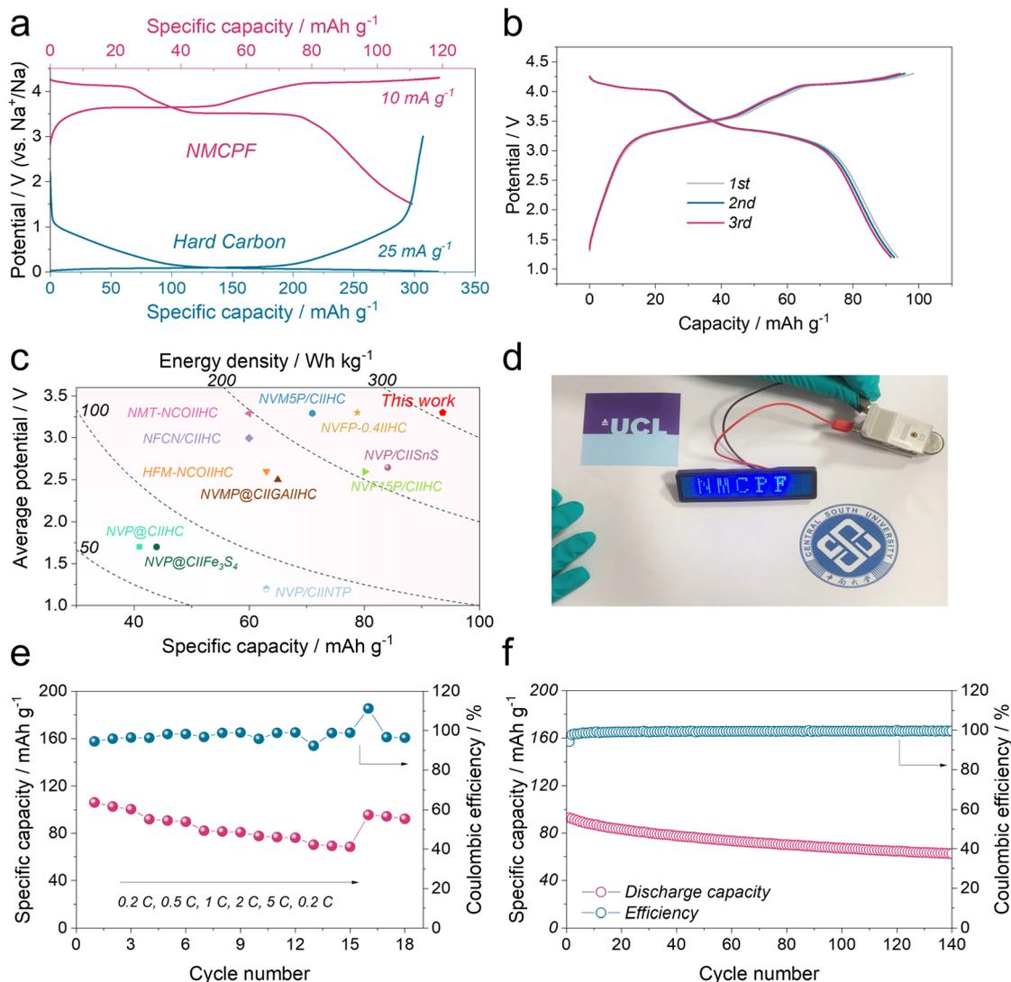
Fig. 5 Electrochemical performances of the HC||NMCPF full cell. (a) Voltage curves of the HC anode and the NMCPF cathode. (b) Charge-discharge profiles of the HC||NMCPF full cell for the initial three cycles at 0.5C ( $1\text{C} = 110\text{ mA g}^{-1}$ ). (c) Comparison of our work with previous reported works. (d) Picture of a LED badge powered by the HC||NMCPF full cell. (e) Rate capability of the full cell. (f) Cycling stability of the full cell at 0.5C.
