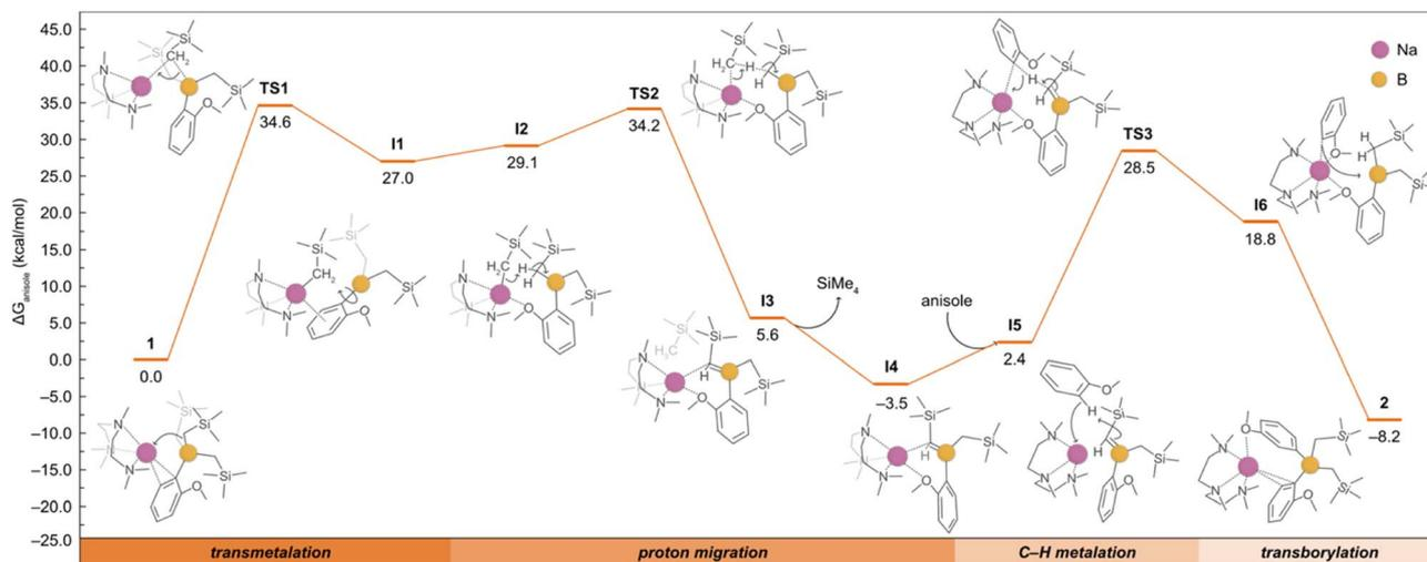
Fig. 4 Gibbs energy profile for the deprotonative borylation of anisole from **1** to afford **2**. Gibbs energies are calculated at the experimental conditions of 353.15 K and 1 atm, in anisole as solvent (see ESI† for details). The bottom bar highlights the four main reaction steps, and the detailed mechanism is shown with the aid of curly arrows.
