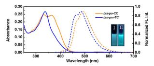
Fig. 5 UV-vis absorption (solid lines) and fluorescence (dashed lines) spectra of *bis-po-CC* and *bis-pm-TC* in dichloromethane ( $c=1.0\times10^{-5}$  M). Photograph showing the fluorescence of *bis-po-CC*(I), and *bis-pm-TC*(II) under 365 nm using a UV lamp (inset).
