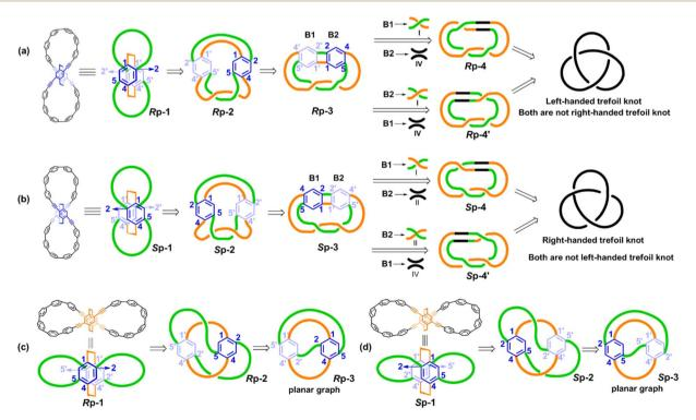
Fig. 2 Topological analyses: (a and b) representative topological transformations of  $R_P$ -bis-pm-TC and  $S_P$ -bis-pm-TC into the left- and right-handed trefoil knot graphs, respectively. (c and d) Representative topological transformation of  $R_P$ -bis-po-CC and  $S_P$ -bis-po-CC into the planar graphs.
