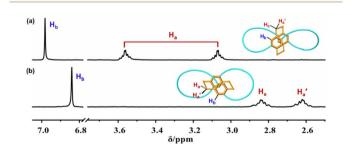
Fig. 3 Comparison of the  $^1$ H NMR spectra (600 MHz, CDCl $_3$ , 298 K) of (a) bis-po-CC and (b) bis-pm-TC.
