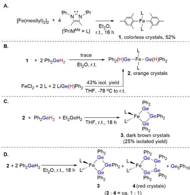
Scheme 4 Synthesis of iron complexes **1**–**4**. (A) Synthesis and isolation of **1**. (B) Two reaction schemes for the synthesis of **2**. (C) Synthesis and isolation of **3**. (D) Synthesis of *ca.* a 1 : 1 mixture of iron complexes **3** and **4**.
