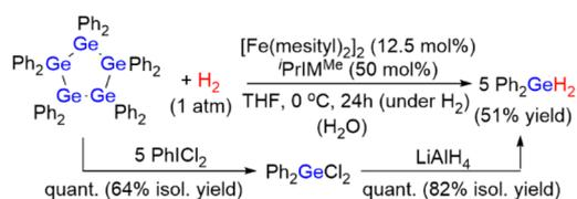
Scheme 3 Regeneration of  $\text{Ph}_2\text{GeH}_2$  from  $(\text{GePh}_2)_5$ .
