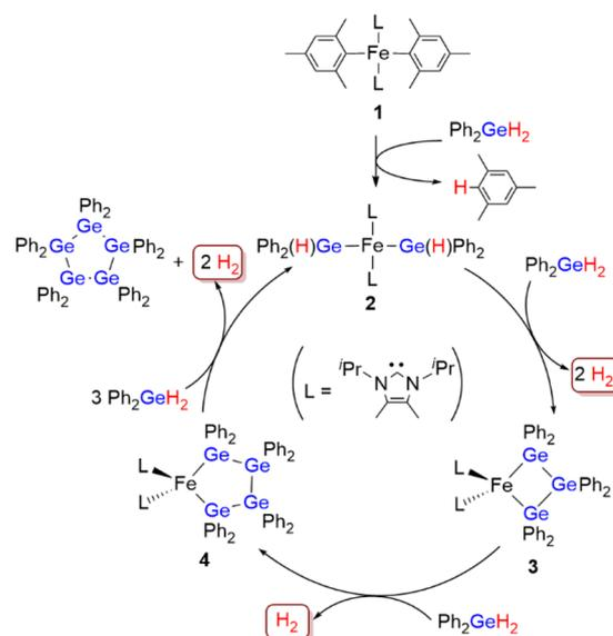
Scheme 5 Plausible reaction mechanism for the sequential production of  $\text{H}_2$  and Ge–Ge bond propagation to afford cyclopentagermane  $(\text{GePh}_2)_5$  *via* the dehydrogenative coupling of  $\text{Ph}_2\text{GeH}_2$  catalyzed by  $[\text{Fe}(\text{mesityl})_2]_2/{}^i\text{PrIM}^{\text{Me}}$ .
