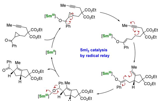
Scheme 5 Schematic catalytic cycle of the  $\text{Sm}^{\text{II}}$ -induced electron transfer followed by cyclization and back electron transfer.<sup>137</sup>
