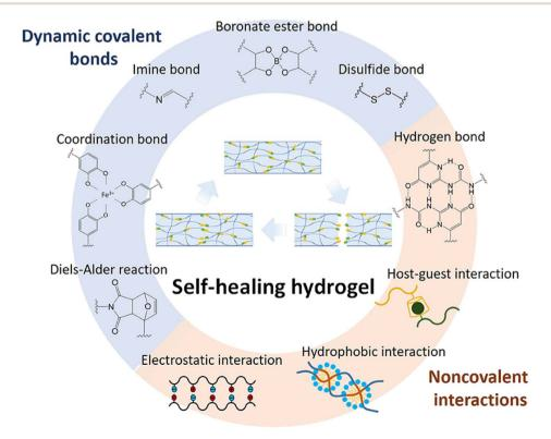
Fig. 4 Summary of self-healing mechanisms employed in hydrogels. <sup>126</sup> This figure has been adapted/reproduced from ref. 126 with permission from *Frontiers in Chemistry*, copyright 2023.
