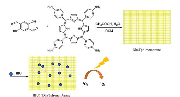
Fig. 8 The preparation of multifunctional antimicrobial IBU@DhaTph-membrane. Reproduced with permission from ref. 81.
