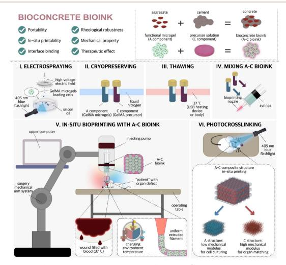
Fig. 2 Train of thought of A-C bioink designing and sketch of the preparing/using method.<sup>34</sup> Reproduced from ref. 34 with permission from the Springer Nature Limited, Copyright@ 2023.
