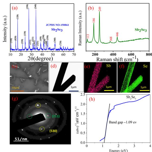
**Fig. 1** Characterization studies of Sb<sub>2</sub>Se<sub>3</sub> NRs: (a) XRD pattern, (b) Raman spectra, (c) scanning electron microscopy image, (d) transmission electron microscopy image, (e and f) FETEM colour mapping of Sb and Se, (g) selected area electron diffraction pattern and (h) Kubelka–Munk plot.
