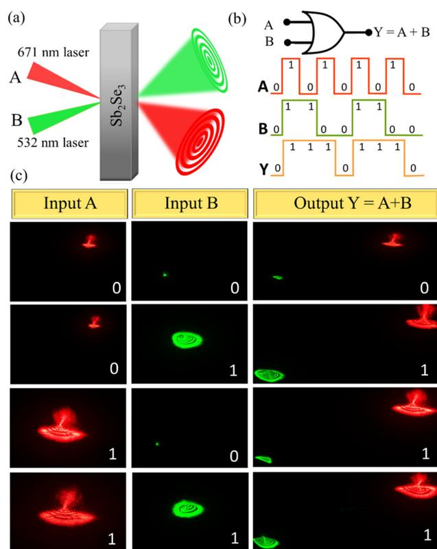
**Fig. 6** All-optical logic application: realization of all-optical modulation by self-phase modulation and demonstration of the OR logic function. (a) Schematic of the light–light modulation system, (b) two input OR gate: input and output waveform of the OR logic operation and (c) experimental results of the OR logic operation with 671 and 532 nm laser beams.
