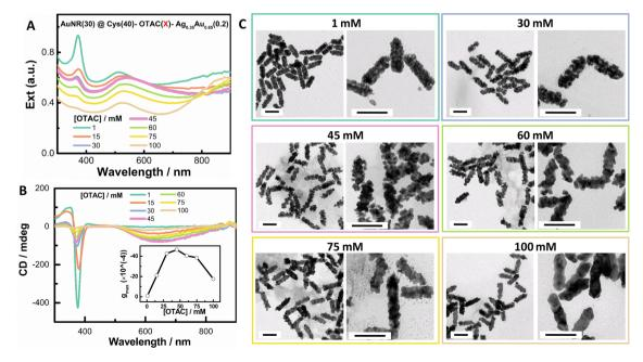
Fig. 3 Effect of OTAC concentration on the growth of the helical shell for AuNR(30)@Cys(40)-OTAC(X)-Ag<sub>0.35</sub>Au<sub>0.65</sub>(0.2). (A) Extinction and (B) CD spectra. Inset in B:  $g_{max}$  vs. OTAC concentration. (C) TEM images. Scale bar: 100 nm.
