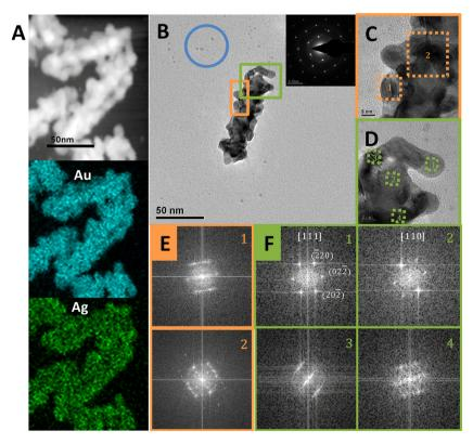
$\textbf{Fig. 5} \quad \text{TEM characterization of } \text{AuNR} (60) @ \text{Cys} (40) - \text{OTAC} (45) - \text{Ag}_{0.35} \text{Au}_{0.65} (0.2). \ \textbf{(A) STEM image and corresponding Au and Ag element mapping and corresponding Au and Corr$ picture. (B) TEM image of one helical nanostructure. Inset: SAED pattern. (C and D) Zoom-in HRTEM images indicated in (B). (E) FFT patterns of marked regions in (C). (F) FFT patterns of marked regions in (D).
