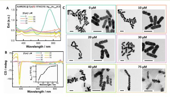
Fig. 2 Effect of Cys concentration on the formation of island helical shells mediated by OTAC (15 mM). (A) Extinction and (B) CD spectra. Inset:  $g_{\text{max}}$ vs. Cys concentration. (C) Typical TEM images of AuNR(30)@Cys(X)-OTAC(15)-Ag<sub>0.35</sub>Au<sub>0.65</sub>(0.2) nanostructures obtained at different Cys concentrations. Scale bar: 100 nm.
