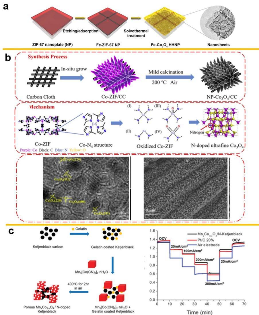
Fig. 11 (a) Metal on  $\text{Co}_3\text{O}_4$  derived from ZIF-67, (reproduced from ref. 203 with permission Copyright © 2020 from Songlin Zhang *et al.*, published by Wiley) (b) N-doped  $\text{Co}_3\text{O}_4$  on Carbon Cloth, (reproduced from ref. 205 with permission Copyright © 2020 Elsevier) (c)  $\text{Mn}_x\text{Co}_{3-x}\text{O}_4$  derived from Prussian blue with high stability in ZABs. (Reproduced from ref. 206 with permission. Copyright © 2016 Wiley-VCH).
