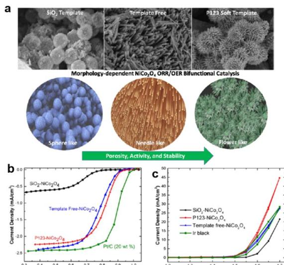
Fig. 10 (a) Morphology and (b) OER and (c) ORR performance of  $\text{NiCo}_2\text{O}_4$  formed by  $\text{SiO}_2$  templated, P123 templated, and template free synthesis.<sup>201</sup> (Reproduced from ref. 201 with permission. Copyright © 2017, American Chemical Society).
