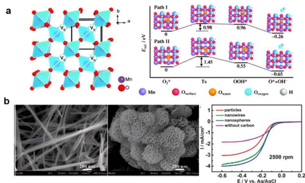
Fig. 7 (a) Oxygen induced MnO<sub>2</sub> (reproduced from ref. 160 with permission. Copyright © 2013 Wiley-VCH) (b) morphology control of MnO<sub>2</sub> and ORR performance (reproduced from ref. 163 with permission. Copyright © 2010, American Chemical Society).
