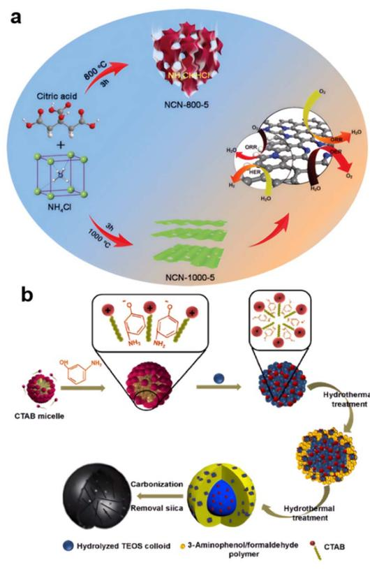
Fig. 4 Templates and evaporation method generating porous (a) NH<sub>4</sub>Cl (reproduced from ref. 109 with permission. Copyright © 2021 Elsevier) (b) silicon and CTAB assisted (reproduced from ref. 112 with permission. Copyright © 2020, Nature).
