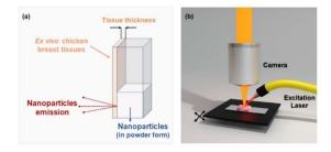
Fig. 3 Schematic representations of the experimental setup used for spectral distortions induced by tissue. (a) Representation of  $ex\ vivo$  tissue disposition and used nanoparticles. (b) Illustration of the experimental system used for spectral distortion of the Yb–Er–Tm CaF<sub>2</sub> NPs induced by  $ex\ vivo$  tissue.
