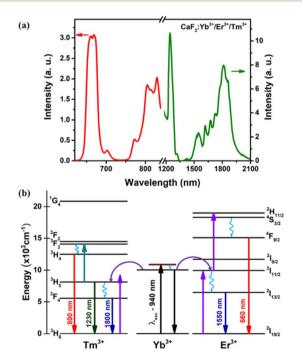
Fig. 5 (a) Emission spectrum of Yb $^{3+}$ /Er $^{3+}$ /Tm $^{3+}$  tri-doped CaF $_2$  NPs under 940 nm excitation at room temperature in the I-BW (red), II-BW (left peak of the green spectrum) and III-BW (right peak of the green spectrum). (b) Simplified energy scheme of the Yb $^{3+}$ , Er $^{3+}$  and Tm $^{3+}$  ions, showing excitation and emission decays (full lines), nonradiative decays (wavy lines), and the energy transfer process (curved lines).
