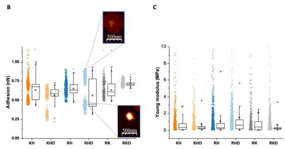
Fig. 3 Mechanical nanoparticles characterization. (A) AFM images of the 6 nanoparticles constructs; on the top are the cationic and at the bottom the coated ones. Heigh scale bar is in nanometres. (B) Adhesion values plot with AFM magnifications of two of the populations of RHD. (C) Young modulus of the polyplexes, as calculated by AFM.
