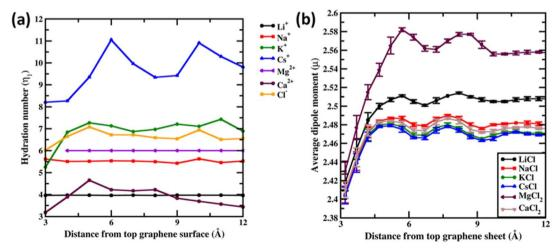
Fig. 5 (a) First hydration number ( $\eta_1$ ) for Li<sup>+</sup>, Na<sup>+</sup>, K<sup>+</sup>, Cs<sup>+</sup>, Mg<sup>2+</sup>, Ca<sup>2+</sup> and Cl<sup>-</sup> ions from 1 M ion–graphene simulations as a function of distance from the graphene surface. (b) Average dipole moment ( $\mu$ ) for water molecules in various 1 M salt solutions discussed in the study. All distances are presented in units of Å. Dipole moments are presented in units of Debye.
