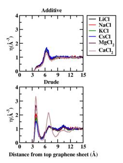
Fig. 4 Number density  $(\eta)$  for Cl<sup>-</sup> as a function of distance from the topmost graphene sheet, from 1 M additive and Drude polarizable FF salt simulations. All distances are presented in units of Å.
