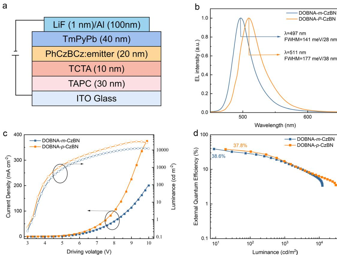
Fig. 3 Device structure and performance of OLEDs. (a) Device configuration. (b) Normalized electroluminescence spectrum. (c) Current density–voltage–luminance curves. (d) EQE–luminance curves.
