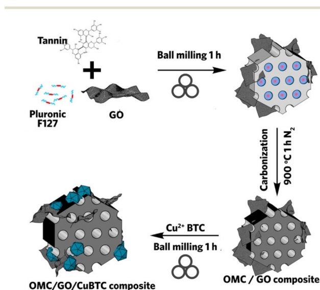
Fig. 7 Schematic procedure of mechanochemically synthesized OMC/GO/CuBTC composite. Reproduced with permission from ref. 97.
