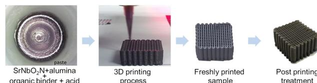
**Fig. 2** (left)  $\text{SrNbO}_2\text{N}$ -containing printing ink prepared by mixing  $\text{SrNbO}_2\text{N}/\text{Al}_2\text{O}_3$  powder, organic binder and acid solution to obtain a printable viscosity; resulting 3D printed monolith freshly printed, dried and thermally treated (viewed from left to right).
