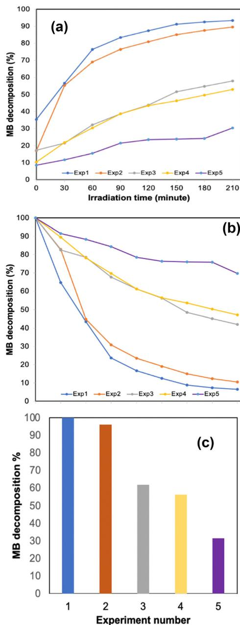
Fig. 4 Methylene blue decomposition % ( $C/C_0 \times 100$ ) over time (a) after post-adsorption equilibrium (MB/3D monolith mixture was kept 30 min in the dark; this was assigned as  $t = 0$ ) and (b) catalytic activity for the entire duration of the experiment (including the adsorption time) (c) the final MB decomposition % with catalyst cycling runs.
