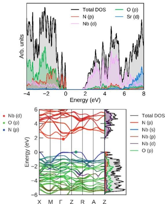
Fig. 12 (left) Total and projected densities of states and (right) band structure for SrNbO<sub>2</sub>N, calculated at the HSE06 level.
