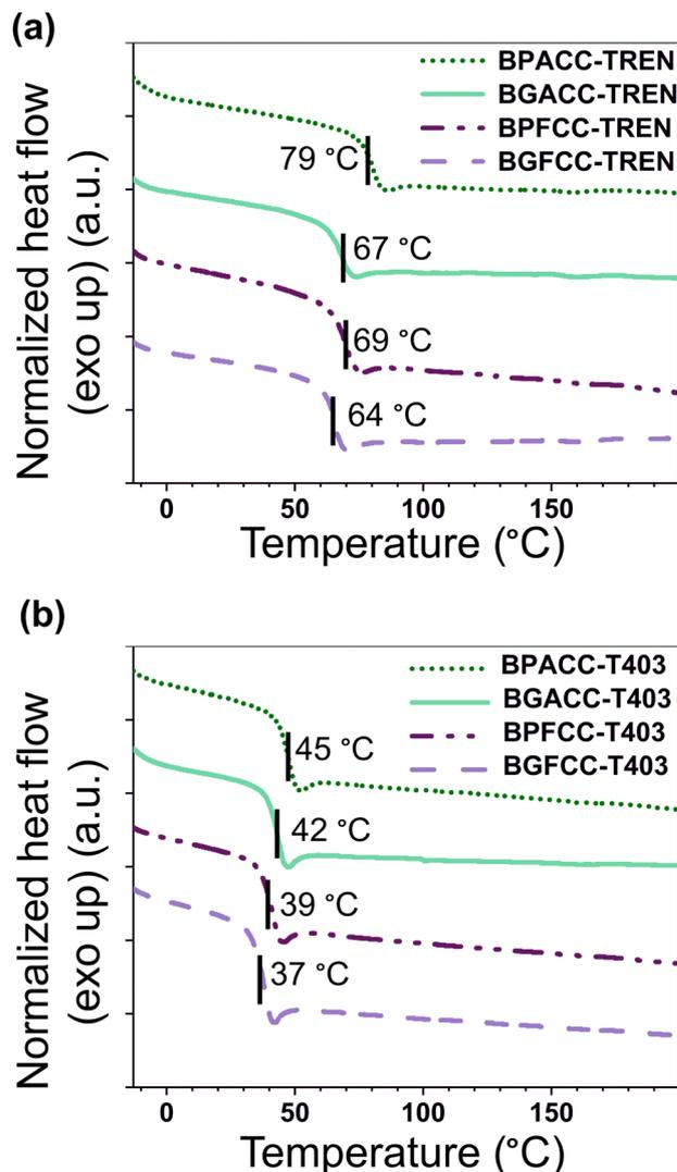
Fig. 1 Representative DSC second heating traces of (a) **TREN**-based and (b) **T403**-based NIPU networks (10 °C min<sup>-1</sup>, N<sub>2</sub>). Curves are shifted vertically for clarity with  $T_g$  values marked on the respective curves. Each tick mark on the y-axis represents a 0.1 W g<sup>-1</sup> increment.
