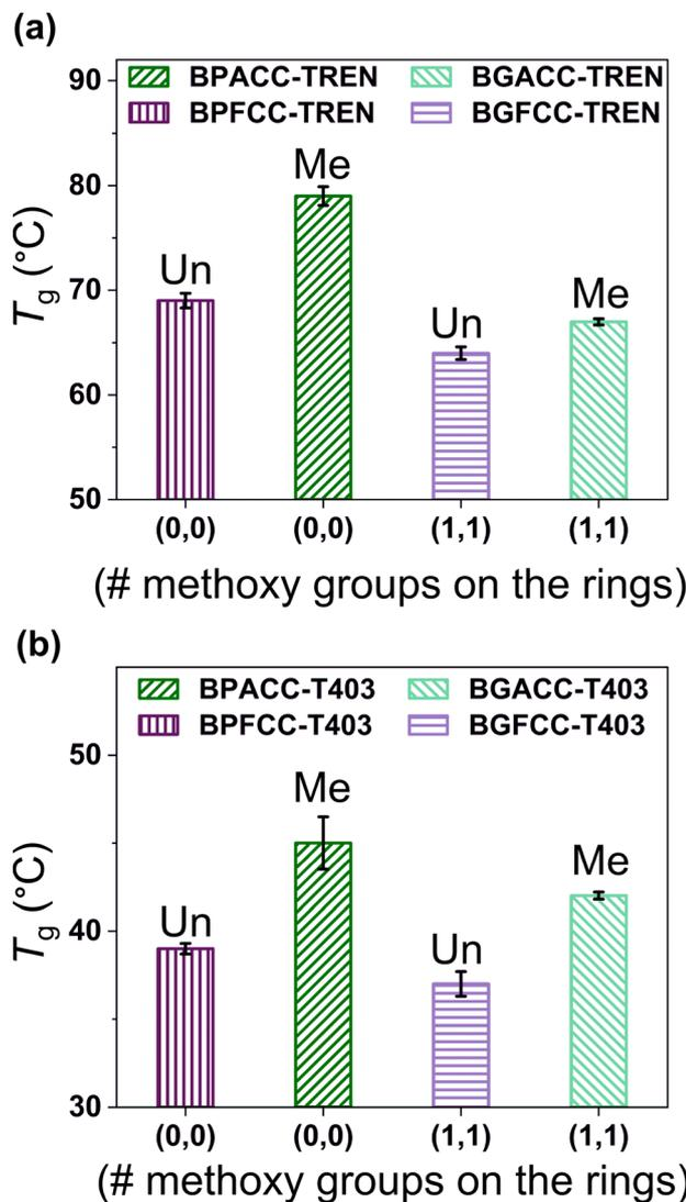
Fig. 2  $T_g$  as a function of the number of methoxy groups on the rings with the type of bridging-carbon substitution as bar labels for (a) TREN-based NIPU networks and (b) T403-based NIPU networks. Error bars indicate standard deviations of the measurements.
