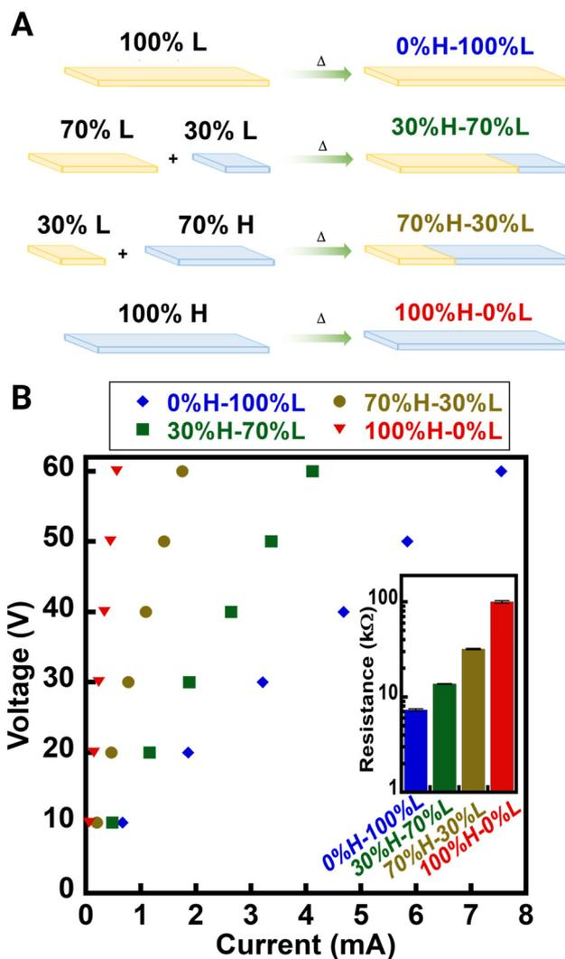
**Fig. 5** (A) Illustration of how custom resistors are achieved *via* healing using IPN-Lin<sub>100</sub>UPy<sub>7.5</sub>FMA<sub>7.5</sub>2.5%CNT and IPN-Lin<sub>100</sub>UPy<sub>7.5</sub>FMA<sub>7.5</sub>1%CNT, (B) Impact of current on custom resistors using current–voltage plots, and the measured resistance (inset) of each resistor.
