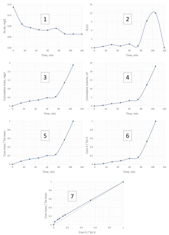
Fig. 5 Example of the drawing of one M(V) curve for Fe<sub>dis</sub> for event 2. The numbers 1–7 indicate the order of drawing each point of the M(V) curve from both the hydrograph and the pollutograph.
