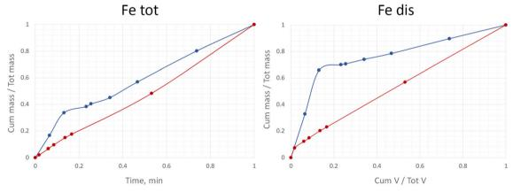
Fig. 6 First flush graphical analysis of the ratio runoff mass fraction and volume fraction for two rainfall events.
