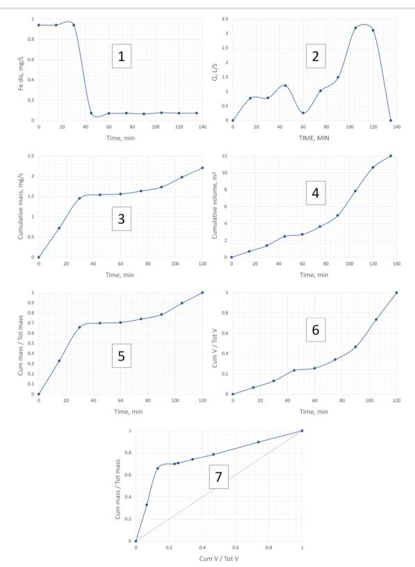
Fig. 4 Example of the drawing of one M(V) curve for Fe<sub>dis</sub> for event 1. The numbers 1–7 indicate the order of drawing each point of the M(V) curve from both the hydrograph and the pollutograph.
