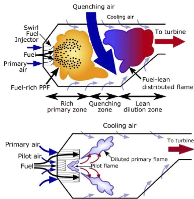
Fig. 3 Sketches of combustion chambers from Bergthorson and Thomson (2015),<sup>40</sup> showing RQL (top) and TAPS lean burn (bottom) combustors.
