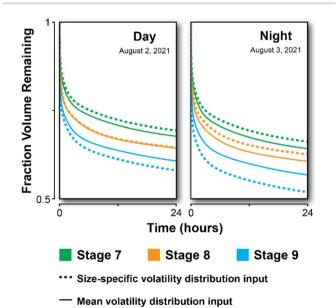
Fig. 4 Simulated evaporation kinetics for size-resolved wildfire organic aerosol using mass spectrometry signal intensity weighted volatility distribution data inputs.
