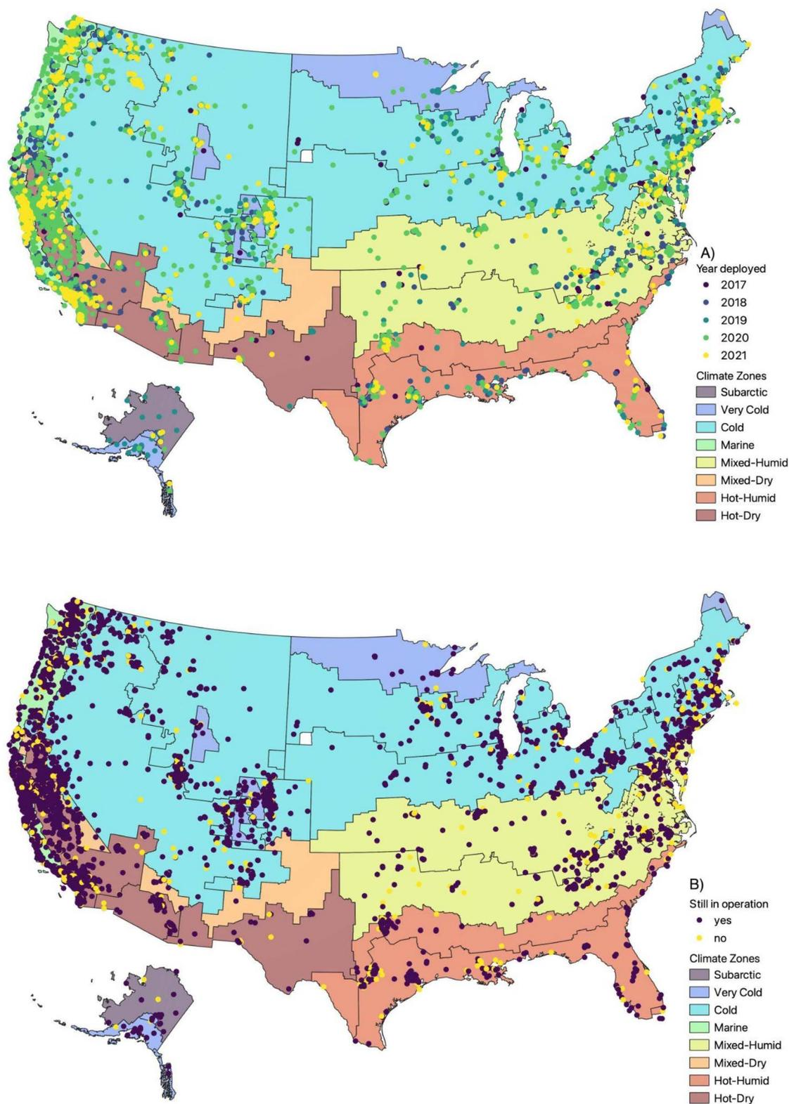
**Fig. 1** The distribution of PurpleAir sensors considered in this analysis (Hawaii is not displayed) depicting (A) the year each sensor was deployed, and (B) if the sensor was removed before 20 July 2021. Climate zones displayed are from the International Energy Conservation Code (IECC) climate zones (<https://codes.iccsafe.org/content/IECC2021P1/chapter-3-ce-general-requirements>, last accessed August 31, 2022).
