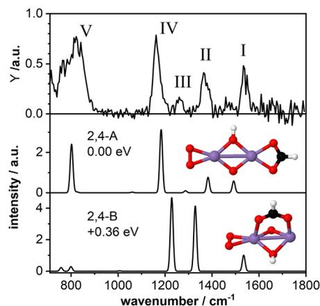
Fig. 4 IR-MPD spectrum (top) of  $\text{Mn}_2\text{O}_4(\text{HCOOH})^+$  together with calculated vibrational spectra of two isomeric structures containing a formate group. Mn, O, C, and H atoms are depicted as purple, red, black, and white spheres. The IR-MPD spectrum has been obtained with reduced IR macropulse fluence to achieve better resolution. The spectrum obtained at higher fluence is shown in Fig. 2.
