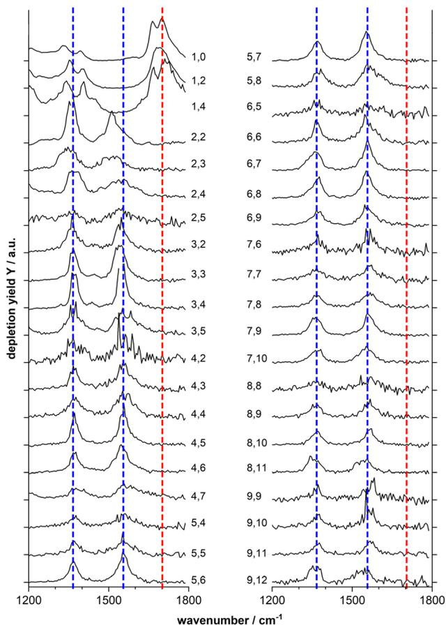
**Fig. 2** IR-MPD spectra of  $\text{Mn}_x\text{O}_y(\text{HCOOH})^+$  complexes (labeled  $x, y$  to the right and left of the spectra, respectively). The blue and red dotted line are drawn to guide the eye. The black tick marks on the  $y$ -axis indicate the zero depletion yield for each spectrum.
