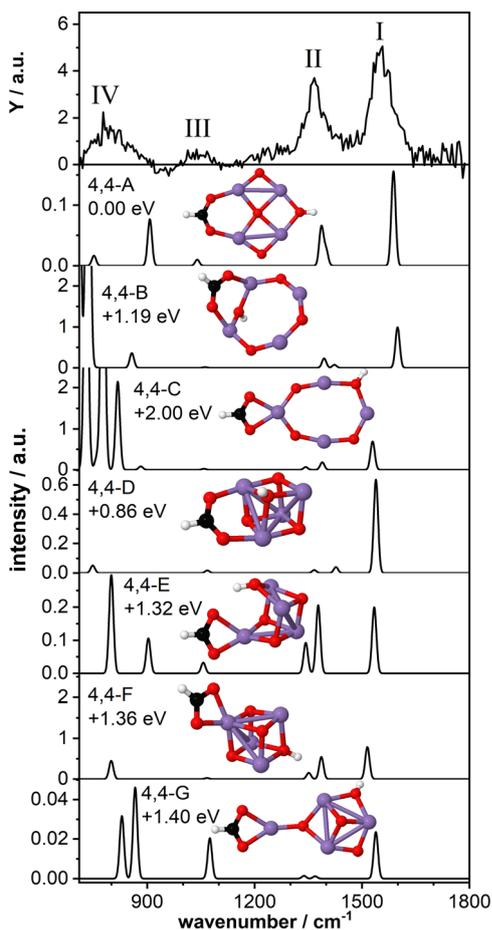
Fig. 5 IR-MPD spectrum (top row) of  $\text{Mn}_4\text{O}_4(\text{HCOOH})^+$  together with calculated vibrational spectra of several 2D and 3D isomeric structures. Mn, O, C, and H atoms are depicted as purple, red, black, and white spheres.
