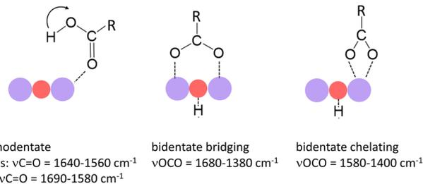
**Fig. 1** Binding modes of small carboxylic acids to manganese oxide clusters and most characteristic vibrational modes.<sup>36,40–42</sup> Purple and red balls indicate Mn and O atoms of the cluster. The left mode indicates the *trans*-configuration; the arrow indicates the position of the H atom in the *cis*-configuration.
