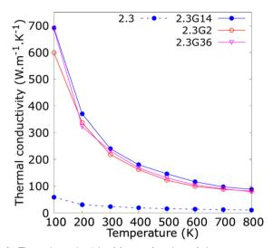
Fig. 4 Thermal conductivity  $(\kappa)$  as a function of the temperature for copper-argon and copper-graphene-argon nanofluids (structures shown in Fig. 2(c)) when the copper nanoparticle has a diameter of 2.3 nm and is covered by 14, 2 and 36 graphene flakes enough to cover the whole nanoparticle surface.
