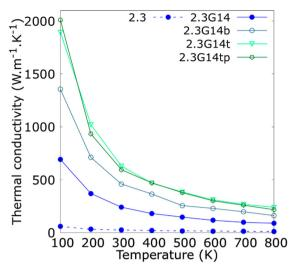
Fig. 5 Thermal conductivity ( $\kappa$ ) as a function of the temperature for copper-argon and copper-graphene-argon nanofluids (structures shown in Fig. 2(d)) when the copper nanoparticle has a diameter of 2.3 nm and is covered with 14 monolayer, bilayer, trilayer and trilayer perpendicular graphene flakes big enough to cover the whole nanoparticle surface.
