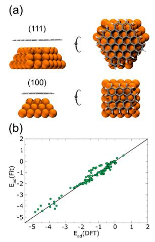
Fig. 1 (a) Side and top views of 2 of 193 nanostructures on several sites, heights, and configurations on the surfaces used to model the flake-Cu NP interaction for the Morse potential fitting. The (111) and (100) faces of the Cu NP were considered, shown at the top and bottom, respectively. (b) Adsorption energies for each one of the 193 nanostructures. DFT and fitted Morse values are compared.
