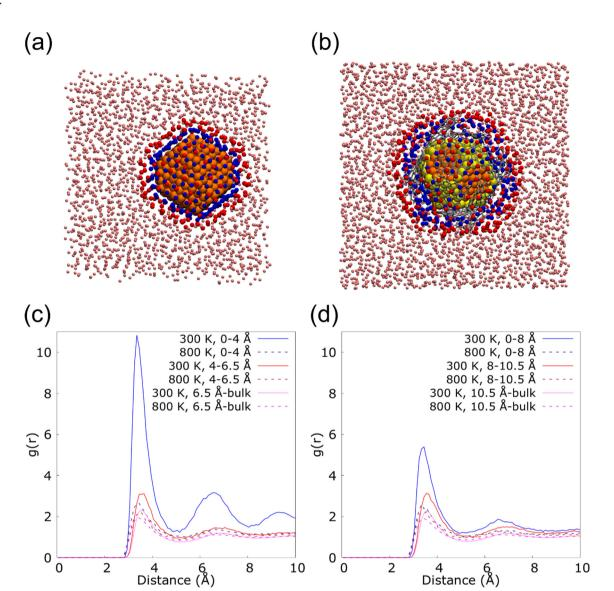
Fig. 6 First (blue) and second (red) argon neighbors of the copper nanoparticle of d = 2.3 nm at 300 K when it is (a) uncapped and (b) capped by 14 graphene flakes big enough to cover the whole nanoparticle surface. Radial distribution function (RDF) calculated at 300 and 800 K for the nanofluids containing the (c) uncapped and (d) capped nanoparticles mentioned above.
