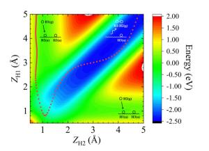
Fig. 2 Two-dimensional energy contour plot for showing the ER and exchange channels (corresponding structures illustrated by insets) as a function of  $Z_{\rm H1}$  (distance between the surface and H1) and  $Z_{\rm H2}$  (distance between the surface and H2). A representative ER trajectory is projected onto this contour plot by red dots. The energy zero is the same as that
