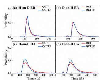
**Fig. 3** Reaction time distributions of direct ER (a and b) and HA (c and d) mechanisms in both H-on-D and D-on-H collisions. The time interval starts when the incident atom enters and it ends when the center mass of the HD molecule leaves the interaction zone, which is defined up to 5.0 Å above the surface.
