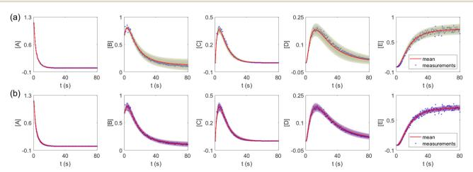
Fig. 3 The (a) VI and (b) HMC results for the five species in the elementary reaction system. Blue dots are the synthetic measurements with 5% of Gaussian noise. The shaded regions indicate 4 standard deviation intervals. Red lines are the mean values of the generated trajectories.
