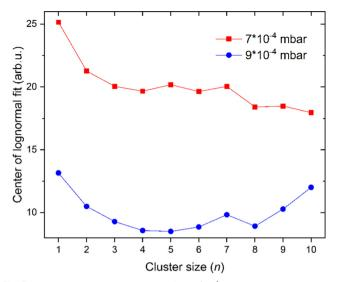
Fig. 3 The cluster size distributions of  $He_mCu_n^+$  that were measured at an evaporation pressure of  $7 \times 10^{-4}$  (red squares) and  $9 \times 10^{-4}$  mbar (blue circles) are fitted with lognormal distributions and the center of these fit functions is plotted against the cluster size n
