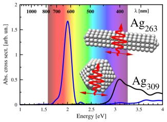
Fig. 1 Optical absorption spectra of the two systems used for illustration in the present paper, the quasi-spherical icosahedral Ag<sub>309</sub> and the nanorod Ag<sub>263</sub>. The arrows indicate the direction of the electric field of the optical excitation in the dynamic case, which is identical to the direction of the electric field applied in the static case. The spectrum of Ag<sub>309</sub> is multiplied by a factor of 5.
