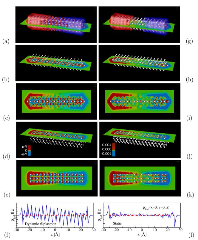
Fig. 3 Representations of the induced densities of an optical excitation at the SPR frequency and as reaction to a static electric field as in Fig. 2 for the nanorod Ag<sub>263</sub>. The color-coded slab representations of the second and the fourth rows are shown from a perpendicular view angle in the third and the fifths rows for better visibility.
