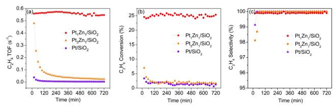
Fig. 7 (a)  $C_2H_4$  TOF s<sup>-1</sup>, (b)  $C_2H_6$  conversion and (c)  $C_2H_4$  selectivity as a function of reaction time (reaction conditions: T = 550 °C,  $C_2H_6 = 18\%$  with balance He. 100 mg catalyst was used for each test. All catalysts were pre-treated with 5% H<sub>2</sub>/He for 30 min at 600 °C before DHE, WHSV = 7.2 h<sup>-1</sup>).
