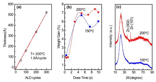
Fig. 1 (a) Growth rate of ZnO ALD at 200 °C with time sequence 0.03-10-0.1-10 s, (b) weight gain as a function of DEZ dose time with time sequence  $t_1$ -200-40-200 s, (c) XRD of the ALD ZnO/SiO<sub>2</sub> sample prepared at 150 °C and 200 °C.
