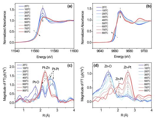
Fig. 5 Pt L<sub>3</sub> edge (a) XANES, (b) EXAFS Fourier transform of Pt/ZnO/SiO<sub>2</sub> during in situ hydrogen reduction at elevated temperatures and their Zn K edge XANES (e) and (d) EXAFS counterparts.
