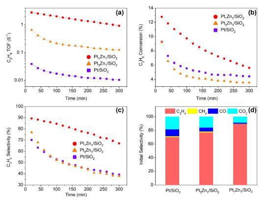
Fig. 8 (a) C<sub>2</sub>H<sub>4</sub> TOF, (b) C<sub>2</sub>H<sub>6</sub> conversion and (c) C<sub>2</sub>H<sub>4</sub> selectivity as a function of reaction time. (d) Initial selectivity of the product gases on the catalysts. (Reaction conditions: T = 550 °C,  $C_2H_6 = 22.3\%$ ,  $O_2 = 1.7\%$ , He = 76%, total flowrate = 50 ml min<sup>-1</sup>. All catalysts were pre-treated with 5%  $H_2/He$  for 30 min at 600 °C before ODHE, initial conversion was at  $\sim$ 10% for all catalysts).
