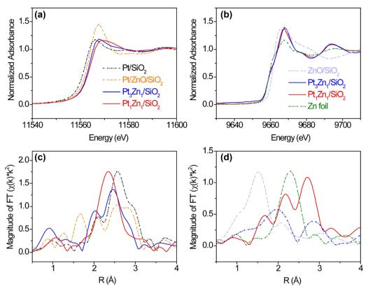
Fig. 3 Pt  $L_3$  edge (a) XANES and (b) EXAFS Fourier transform of Pt/SiO<sub>2</sub>, Pt<sub>1</sub>Zn<sub>1</sub>/SiO<sub>2</sub>, Pt<sub>3</sub>Zn<sub>1</sub>/SiO<sub>2</sub>, Zn K edge (c) XANES and (d) EXAFS Fourier transform of Zn, ZnO/SiO<sub>2</sub>, Pt<sub>3</sub>Zn<sub>1</sub>/SiO<sub>2</sub>, and Pt<sub>3</sub>Zn<sub>1</sub>/SiO<sub>2</sub>.
