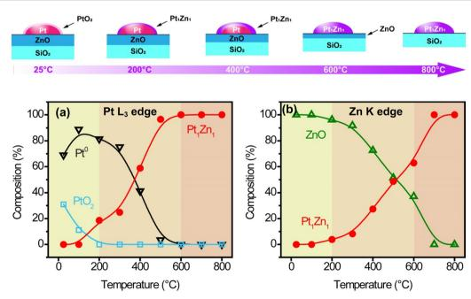
Fig. 6 (a) Scheme of surface species evolution, and XANES linear combination fitting (LCF) of (b) Pt L<sub>3</sub> and (c) Zn K edges.
