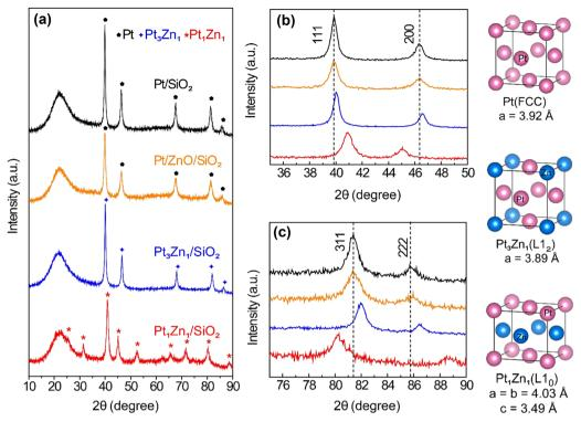
Fig. 2 (a) XRD patterns of Pt/SiO<sub>2</sub>, pre-catalyst Pt/ZnO/SiO<sub>2</sub>, Pt<sub>3</sub>Zn<sub>1</sub>/SiO<sub>2</sub> and Pt<sub>1</sub>Zn<sub>1</sub>/SiO<sub>2</sub>. Detailed scans of XRD patterns of the four samples between (b)  $35-50^{\circ}$  and (c)  $75-90^{\circ}$ .
