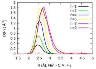
Fig. 7 Na $^+$ (H<sub>2</sub>)<sub>n</sub> radial distributions, normalized to the number of H<sub>2</sub> molecules, for several cluster sizes. The closing shell at n = 8, can be noticed by the small bump that can be appreciated for n = 9.
