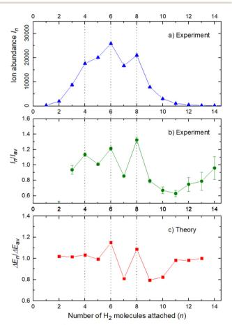
Fig. 5 Data for  $Na^+(H_2)_n$ . Panel a: experimental ion abundance versus size, n. Panel b: experimental ion abundance  $I_n$  divided by its local average,  $I_{\rm av}$ . Panel c: evaporation energy  $\Delta E_n$  calculated with the rigid rotor model DMC, divided by its local average  $\Delta E_{\rm av}$ . Note the similarity of the data in panels b and c.
