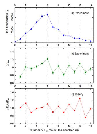
Fig. 6  $Na_2^+(H_2)_n$ . Panel a: experimental ion abundance versus size, n. Panel b: experimental ion abundance  $I_n$  divided by its local average,  $I_{av}$ Panel c: evaporation energy  $\Delta E_n$  calculated with the rigid rotor model DMC, divided by its local average  $\Delta E_{\rm av}$ . Note the similarity of the data in panels b and c.
