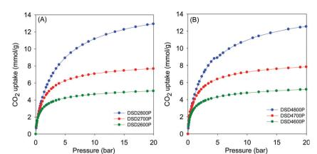
CO<sub>2</sub> uptake isotherms of carbons directly compactivated from sawdust (SD) at 600, 700 or 800 °C, and PO/SD ratio of 2 (A) or 4 (B).
