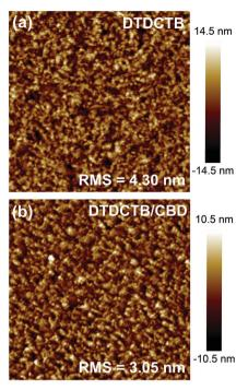
Fig. 3 Surface morphology characterization using AFM height images of (a) DTDCTB and (b) DTDCTB/CBD sublimated films (scan area:  $3.0 \ \mu m \times 3.0 \ \mu m$ ).
