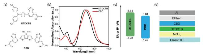
Fig. 1 (a) Molecular structures of the donor DTDCTB and the acceptor CBD. (b) UV-vis-NIR absorption spectra. (c) EA and IP of the DTDCTB and CBD films and (d) device structure of the VD-SMSCs based on DTDCTB and CBD
