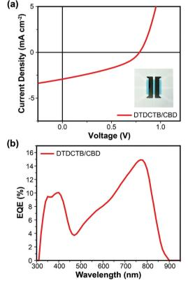
Fig. 2 (a) J-V characteristics and (b) EQE curve for the optimal VD-SMSC based on DTDCTB and CBD under AM 1.5G (100 mW cm<sup>-2</sup>) illumination. The inset graph in (a) is a photograph of the optimal device and the effective area is 0.09 cm<sup>2</sup>.
