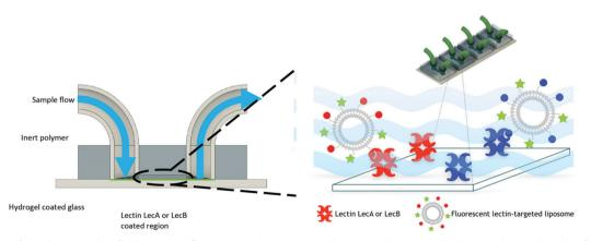
Fig. 3 Concept of the in vitro microfluidic device. Fluorescent lectin-targeted liposomes interact with the proteins LecA or LecB that have been covalently immobilized on the glass surface. The liposomes are retained on the surface due to their specific ligand-lectin interaction and targeting was quantified by microscopy
