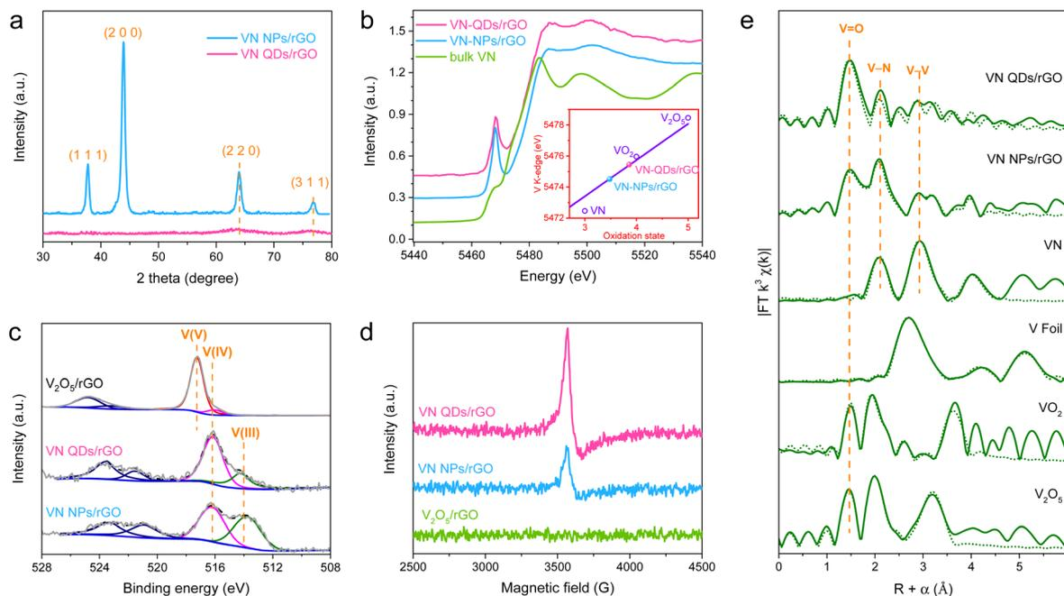
Fig. 2 Characterization of the phase, electronic and coordinate structure of VN QDs/rGO. (a) XRD patterns, (b) V K-edge XANES spectra, (c) high-resolution XPS curves at the V 2p level and (d) ESR spectra of the indicated samples, and (e) FT-EXAFS curves of the samples.
