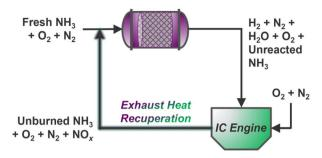
Scheme 2 Steady-state intensified  $NH_3$ -ATR and  $NO_x$ -EGR concept with continuous mass and heat recycling to an ATR monolith inlet.
