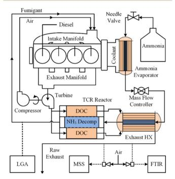
Fig. 3 On-board anhydrous  $NH_3$  thermal reforming reactor and heat exchangers for a diesel/ $NH_3$  dual-fuel tractor engine and exhaust system.<sup>13</sup> Reproduced with publisher permission from ref. 13.
