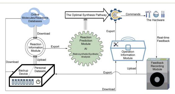
Fig. 4 The configuration of the software includes four parts: the reaction information module, reaction prediction module, reaction operation information module, and feedback recording module.
