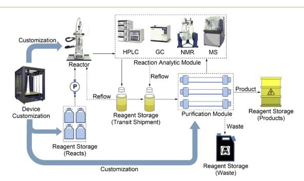
Fig. 3 The configuration of the hardware includes five modules: reagent storage modules, reactors, the reaction analytic module, the purification module, and the device customization module.
