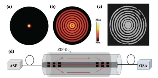
Fig. 13 (a) Optical power distribution of the fundamental mode ( $LP_{01}$ , core mode) and (b) higher-order mode ( $LP_{08}$ , cladding mode); (c) near-field image of the  $LP_{08}$  mode pattern obtained with an infrared camera; (d) schematic diagram of the proposed fibre interferometer with cascaded LPFGs. ASE: amplified spontaneous emission light source; OSA: optical spectrum analyzer.<sup>119</sup>
