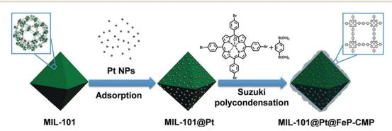
Fig. 7 Illustration of the preparation of MIL-101@Pt@FeP-CMP. Reproduced with permission from ref. 95. Copyright (2018) Wiley-VCH.
