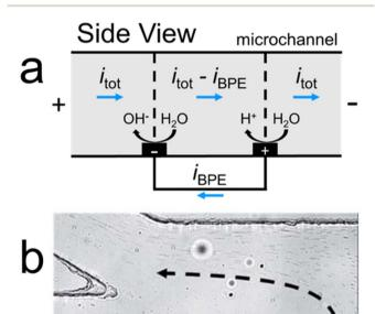
Fig. 4 (a) Schematic illustration of ionic current variations caused by BPEs. Adapted with permission from ChemElectroChem, 2022, 9, e202200251 (Copyright © 2022 WILEY-VCH Verlag GmbH & Co. KGaA, Weinheim). (b) Optical micrograph of a bifurcated microchannel during an electrochemical microplastic separation experiment in buffer-free solution. Adapted from Chem. Sci., 2021, 12, 13744-13755 (copyright © 2022 Royal Society of Chemistry).
