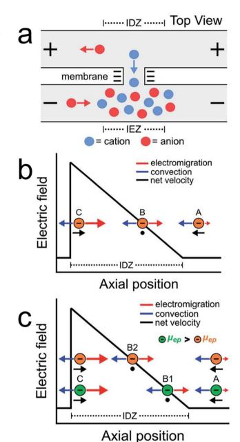
Scheme 1 (a) Representation of a permselective nanochannel connecting two microfluidic channels. (b) Schematic illustration of an electric field gradient in a microchannel and its effect on a single charged ion. (c) Same as (b), but for two ions having different mobilities. Adapted and reprinted from *Chem. Sci.*, 2020, **11**, 5547–5558 (Copyright © 2020 Royal Society of Chemistry).
